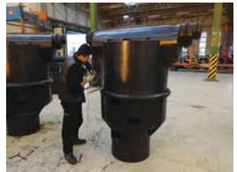
Extruder welding method procedure includes preheating using welding rod and spreading the molten state material on the welding area at a certain speed by applying pressure.
