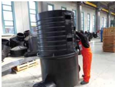
Manual extruder melts the welding rod to join the surfaces together.
