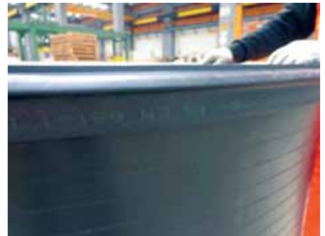
Upon spreading liquid soap in conical top piece seal groove and seal surface, two pieces are joined.
